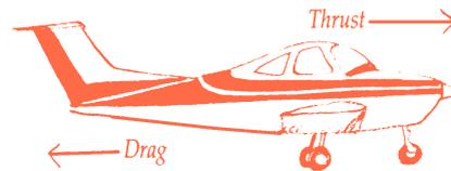
When thrust is greater than drag, during takeoff, for instance, the airplane's speed increases. When thrust and drag are equal, the airplane maintains the same speed. Whenever drag is greater than thrust, the plane slows down.
